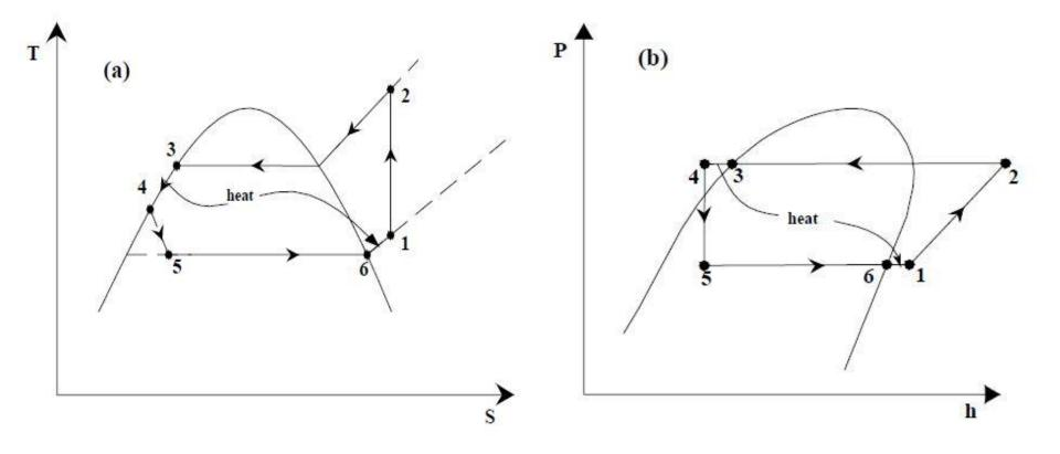
$$\dot{Q}_{LSHX} = \dot{m}_r (h_3 - h_4) = \dot{m}_r (h_1 - h_6)$$
